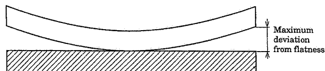
Annex 4 Figure 3 Measurement of flatness
